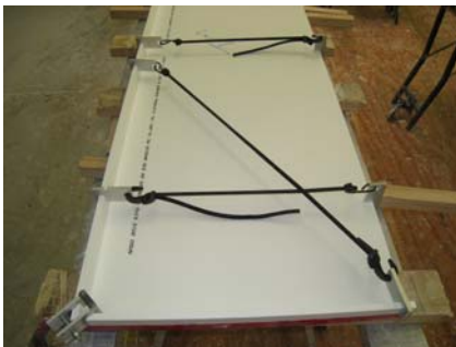
Corner & Edge Clamps in use on v-groove top
